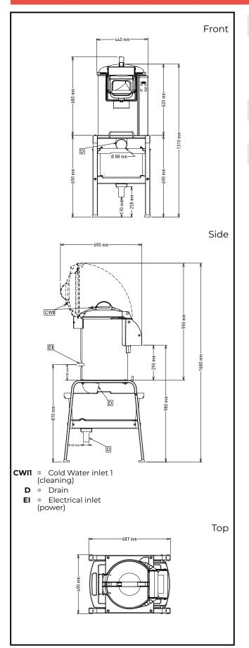
Electric Supply voltage: 603509 (DT10E1) 220-240 V/1N ph/50/60 Hz 200-240/380-440 V/3 603510 (DT10E324) ph/50/60 Hz Electrical power max: 0.37 kW 0.37 kW **Total Watts:** Capacity: Performance (up to): 160 kg/hour Capacity: 10 litres Key Information: External dimensions, Width: 440 mm External dimensions, 690 mm Depth: External dimensions, Height: 680 mm **Shipping weight:** 603509 (DT10E1) 47 kg
